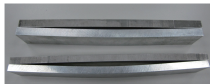
图4 大厚度铝合金板激光喷丸成形效果 Fig.4 Laser peen forming under pre-loading
