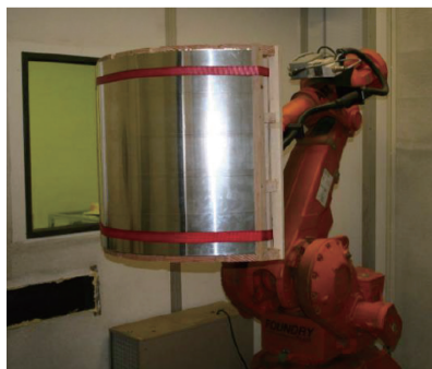
(a) 激光喷丸成形试验
